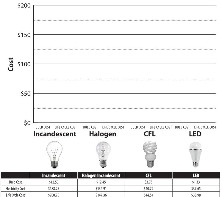
Note: Bulb cost reflects the number of bulbs needed to produce 25,000 hours of light, which is the lifespan of one LED bulb. To produce the same amount of light, it would take 25 incandescent bulbs and 2.5 CFL bulbs.
