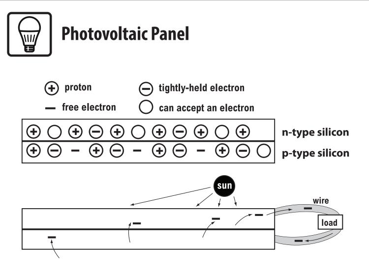
**Photovoltaic** comes from the words *photo*, meaning light, and *volt*, a measurement of electricity. Photovoltaic cells are also called **PV cells** or **solar cells** for short. You are probably familiar with photovoltaic cells. Solar-powered toys, calculators, watches, lighting, and roadside telephone call boxes all use solar cells to convert sunlight into electricity.
